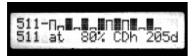
Graphic Display of 16 Slots with a numeric readout of the first displayed slot
